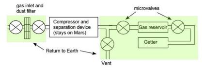
First it uses the getter to remove evolved gases from the container wall. Then it closes one microvalve and opens another to get an atmospheric sample. Finally it closes both microvalves to the gas container and opens the vent to run more atmosphere through the compressor to collect dust in the filter
