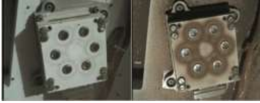
Figure 43: MAHLI images of the REMS UV Sensor on sols 36 (left) and 1314 (right) of the MSL mission. The circular patterns of dust are caused by circular magnets around the UV sensors which attract the dust. The magnets help to keep the sensors free of dust.
