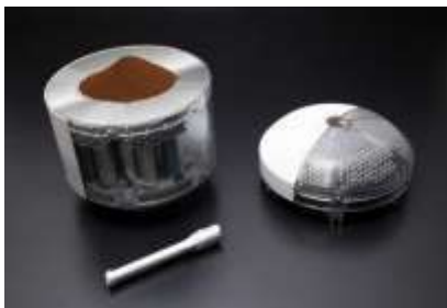
Figure 45: Added proposal for extra dust sample to concept design for the Orbiting Sample Container
