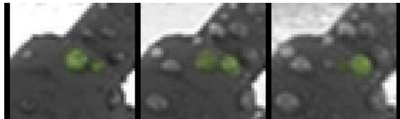
Figure 33 Possible droplets on the legs of the Phoenix lander - they appeared to merge and sometimes fall off. In this sequence of frames, the rightmost of the two droplets - highlighted in green on this black and white image - grows and seems to do so by taking up the water from its companion to the left, which shrinks (Gronstall, 2014)
