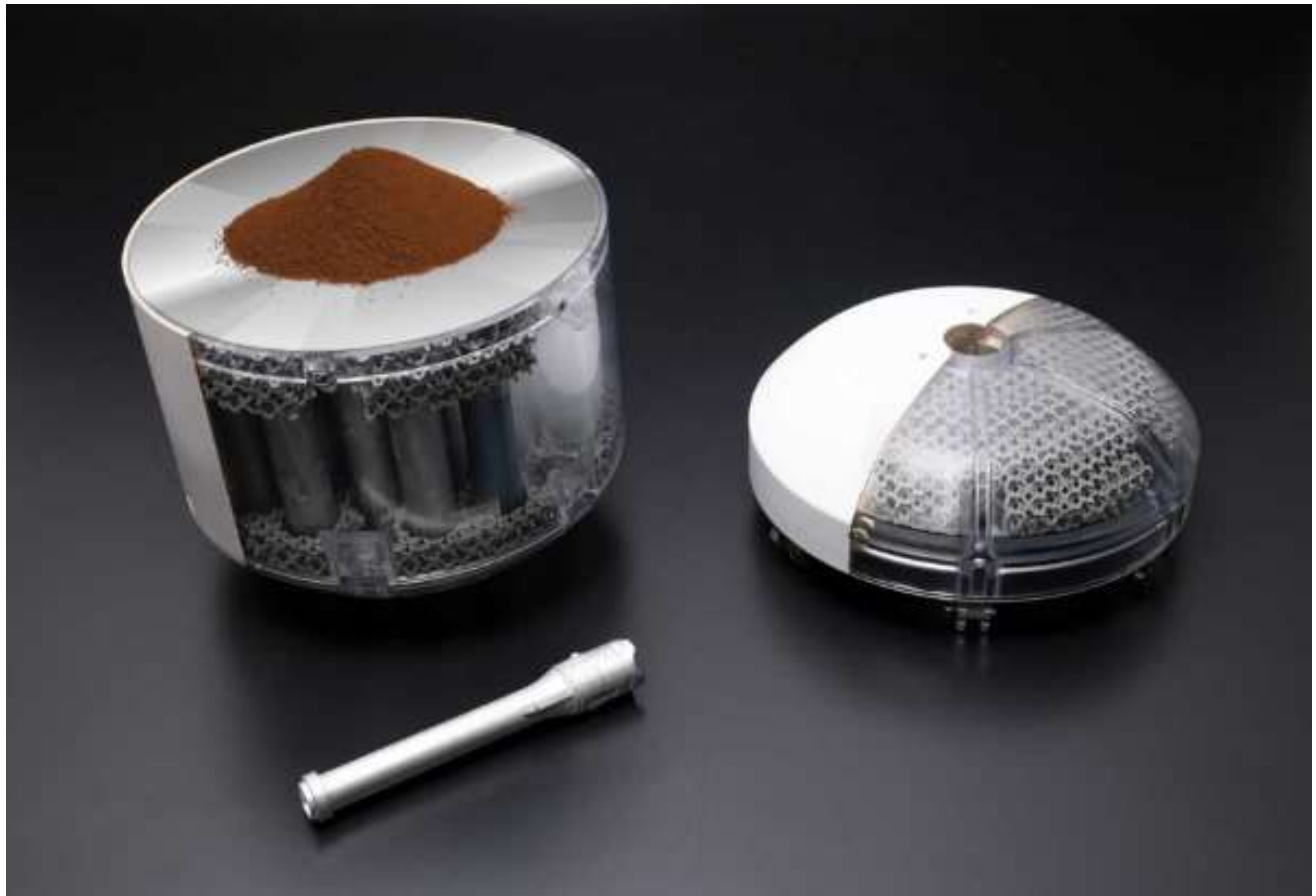
Figure 45: Added proposal for extra dust sample to concept design for the Orbiting Sample Container
